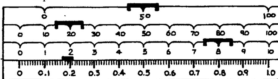
To read the value on the beam, add the largest weight (50g) to the next three (20g, 8g and 0.19g)
