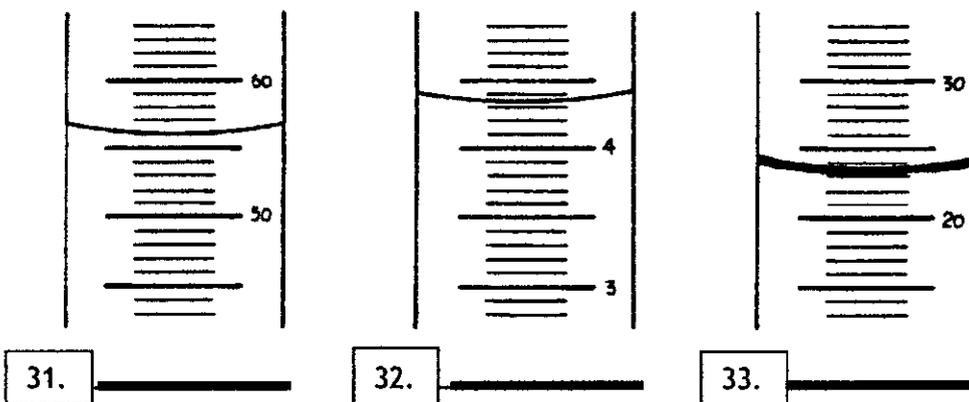
When determining the amount of liquid in a graduated cylinder, sight along the bottom of the curved line called the **meniscus** formed at the surface of the liquid.
